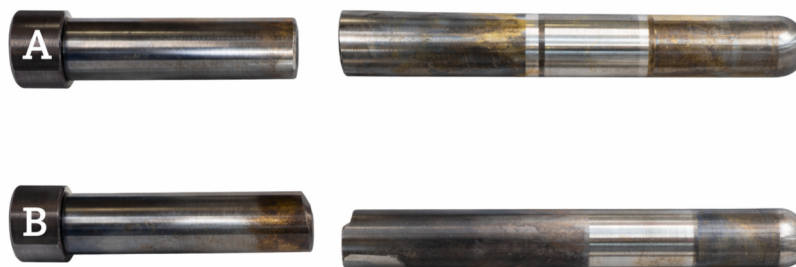
Fig. 1. Examples of brass-tube extrusion mandrels failed by brittle fracture.
